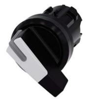
Selector switch, illuminable, 22 mm, round, plastic, white, selector switch, long, 2 switch positions O-I, latching, actuating angle 90°, 10:30h/13:30h Z=50-unit packaging
