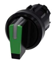
Selector switch, illuminable, 22 mm, round, plastic, green, selector switch, short, 3 switch positions I>O<II, momentary contact on the left, latching on the right, actuating angle  $2x45^{\circ}$ , 10:30h/12h/13:30h Z=50-unit packaging
