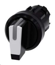
Selector switch, illuminable, 22 mm, round, plastic, white, selector switch, short, 3 switch positions I>O<II, momentary contact type, actuating angle 2x45°, 10:30h/12h/13:30h, with laser labeling, upper case and lower case, always upper case at beginning of line
