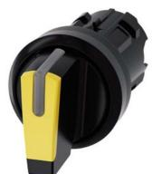
Selector switch, illuminable, 22 mm, round, plastic, yellow, selector switch, short, 3 switch positions I-O-II, latching, actuating angle  $2x45^{\circ}$ , 10:30h/12h/13:30h, with laser labeling, lower case
