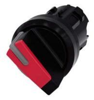
Selector switch, illuminable, 22 mm, round, plastic, red, selector switch, short, 2 switch positions O-I, latching, actuating angle 90°, 10:30h/13:30h, with laser labeling, inscription or symbol Customer-specific selection with SIRIUS ACT configurator (CIN)
