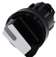
Selector switch, illuminable, 22 mm, round, plastic, white, selector switch, short, 2 switch positions O<I, momentary contact type, Actuating angle 45°, 10:30h/12h Z=50-unit packaging
