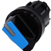
Selector switch, illuminable, 22 mm, round, plastic, blue, selector switch, short, 2 switch positions O<I, momentary contact type, Actuating angle 45°, 10:30h/12h, with laser labeling, inscription or symbol Customer-specific selection with SIRIUS ACT configurator (CIN)
