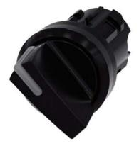
Illuminable selector switch, 22 mm, round, plastic, black, Selector switch short, 2 switch positions O<I, momentary contact type, Actuating angle 45°, 10:30/12, Z=50-unit packaging
