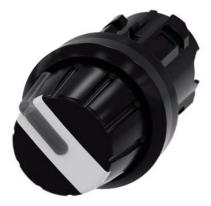
Selector switch, illuminable, 22 mm, round, plastic, white, Rotary knob, 2 switch positions O-I, latching, actuating angle 90°, 10:30h/13:30h, with laser labeling, upper case and lower case, always upper case at the beginning of the word
