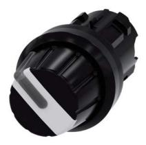
Selector switch, illuminable, 22 mm, round, plastic, white, Rotary knob, 2 switch positions O-I, latching, actuating angle  $90^{\circ}$ , 10:30h/13:30h, with laser labeling, upper case
