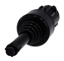
Coordinate switch, 22 mm, round, plastic, black, 2 switch positions, vertical latching, with mechanical interlocking, Z=50-unit packaging
