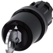
Key-operated switch IKON, 22 mm, round, plastic, lock number 360012K1, with 2 keys, 3 switch positions I>O<II, momentary contact type, actuating angle 2x45°, 10:30h/12h/13:30h, key removal O, with laser labeling, upper case and lower case, always upper case at beginning of line
