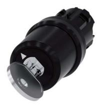
Key-operated switch BKS, 22 mm, round, plastic, lock No. E9 (VW), without key, 2 switch positions O-I, latching, actuating angle  $90^\circ$ , 10:30h/13:30h, key removal O+I, with laser labeling, upper case and lower case, always upper case at beginning of line
