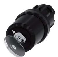
Key-operated switch BKS, 22 mm, round, plastic, Lock No. E9 (VW), without key, 2 switch positions O-I, latching, actuating angle 90°, 10:30h/13:30h, Key removal O+I Z=50-unit packaging
