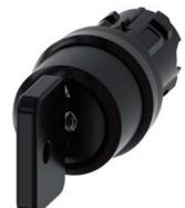
Key-operated switch O.M.R, 22 mm, round, plastic, lock number 73034, black, with 2 keys, 3 switch positions I-O-II, latching, actuating angle 2x45°, 10:30h/12h/13:30h, key removal O, with laser labeling, upper case and lower case, always upper case at the beginning of the word
