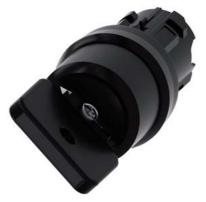
Key-operated switch O.M.R, 22 mm, round, plastic, lock number 73034, black, with 2 keys, 2 switch positions O-I, latching, actuating angle 90°, 10:30h/13:30h, key removal O+I, with laser labeling, lower case
