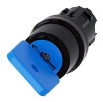
Key-operated switch O.M.R, 22 mm, round, plastic, lock number 73038, blue, with 2 keys, 2 switch positions O-I, latching, actuating angle 90°, 10:30h/13:30h, key removal O+I, with laser labeling, inscription or symbol Customer-specific selection with SIRIUS ACT configurator (CIN)
