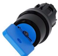
Key-operated switch O.M.R, 22 mm, round, plastic, lock number 73038, blue, with 2 keys, 2 switch positions O<I, momentary contact type, Actuating angle 45°, 10:30h/12h, key removal O, with laser labeling, inscription or symbol Customer-specific selection with SIRIUS ACT configurator (CIN)
