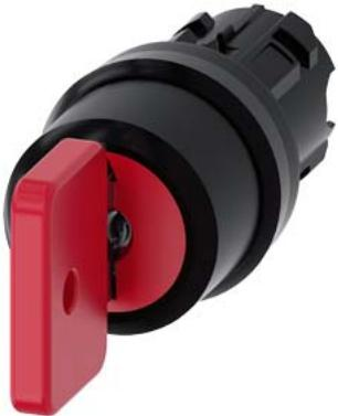
Key-operated switch O.M.R, 22 mm, round, plastic, lock number 73037, red, with 2 keys, 3 switch positions I>O<II, momentary contact type, actuating angle 2x45°, 10:30h/12h/13:30h, key removal O, with laser labeling, upper case and lower case, always upper case at the beginning of the word
