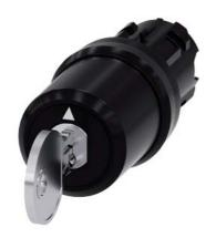
Key-operated switch BKS, 22 mm, round, plastic, lock number S1, with 2 keys, 3 switch positions I-O<II, left latching, right momentary contact type, actuating angle 2x45°, 10:30h/12h/13:30h, key removal O+I, with laser labeling, inscription or symbol Customer-specific selection with SIRIUS ACT configurator (CIN)
