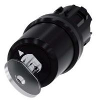
key-operated switch Siemens, 22 mm, round, plastic, lock no. LSG1, with 2 keys, 2 switch positions O-I, latching, actuating angle  $90^\circ,\,10:30h/13:30h,$  key removal O, with laser labeling, upper case
