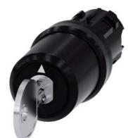
key-operated switch Siemens, 22 mm, round, plastic, lock number SSG10, with 2 keys, 3 switch positions I-O<II, left latching, momentary contact type on the right, actuating angle  $2x45^{\circ}$ , 10:30h/12h/13:30h, key removal O Z=50-unit packaging
