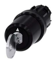
key-operated switch Siemens, 22 mm, round, plastic, lock number SSG10, with 2 keys, 3 switch positions I-O-II, latching, actuating angle 2x45°, 10:30h/12h/13:30h, key removal II, with laser labeling, upper case and lower case, always upper case at the beginning of the word
