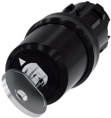
key-operated switch Siemens, 22 mm, round, plastic, lock number SSG10, with 2 keys, 2 switch positions O-I, latching, actuating angle 90°, 10:30h/13:30h, key removal O, with laser labeling, inscription or symbol customer-specific selection with SIRIUS ACT configurator (CIN)
