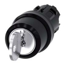
RONIS key-operated switch, 22 mm, round, plastic, lock number SB30, with 2 keys, 3 switch positions I-O-II, latching, actuating angle 2x45°, 10:30h/12h/13:30h, Key removal II, possible special locks: SB31, 421, 455, with laser labeling, lower case
