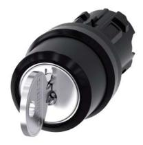
RONIS key-operated switch, 22 mm, round, plastic, lock number SB30, with 2 keys, 3 switch positions I-O-II, latching, actuating angle 2x45°, 10:30h/12h/13:30h, Key removal I+O+II, possible special locks: SB31, 421, 455, with laser labeling, upper case and lower case, always upper case at beginning of line
