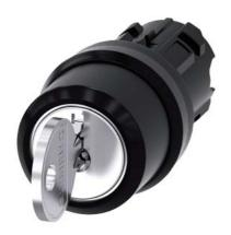
RONIS key-operated switch, 22 mm, round, plastic, lock number SB30, with 2 keys, 3 switch positions I-O-II, latching, actuating angle 2x45°, 10:30h/12h/13:30h, key removal O, possible special locks: SB31, 421, 455, with laser labeling, inscription or symbol Customer-specific selection with SIRIUS ACT configurator (CIN)
