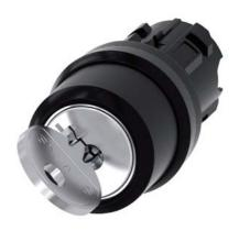
RONIS key-operated switch, 22 mm, round, plastic, lock number SB30, with 2 keys, 2 switch positions O-I, latching, actuating angle 90°, 10:30h/13:30h, key removal O+I, possible special locks: SB31, 421, 455, with laser labeling, lower case
