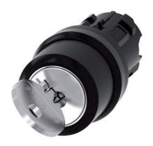
RONIS key-operated switch, 22 mm, round, plastic, special lock, with 2 keys, 2 switch positions O-I, latching, actuating angle 90°, 10:30h/13:30h, key removal O+I, possible special locks: SB31, 421, 455
