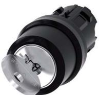
RONIS key-operated switch, 22 mm, round, plastic, lock number SB30, with 2 keys, 2 switch positions O-I, latching, actuating angle 90°, 10:30h/13:30h, key removal O, possible special locks: SB31, 421, 455, with laser labeling, lower case
