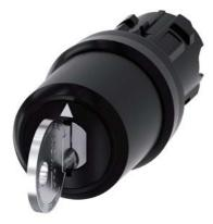
Key-operated switch IKON, 22 mm, round, plastic, lock number 360012K1, with 2 keys, 3 switch positions I>O<II, momentary contact type, actuating angle 2x45°, 10:30h/12h/13:30h, key removal O, with laser labeling, inscription or symbol Customer-specific selection with SIRIUS ACT configurator (CIN)
