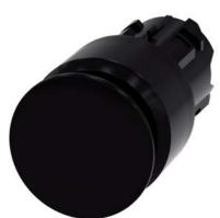
Mushroom pushbutton, 22 mm, round, plastic, black, 30 mm, latching, pull-tounlatch mechanism, with laser labeling, upper case and lower case, always upper case at the beginning of the word
