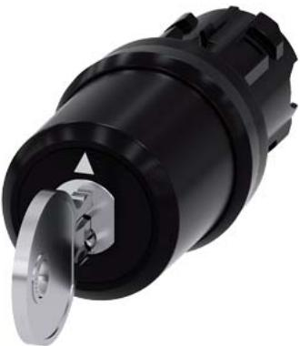
Key-operated switch BKS, 22 mm, round, plastic, Lock No. E2 (VW), without key, 3 switch positions I-O-II, latching, actuating angle 2x45°, 10:30h/12h/13:30h, Key removal I+O+II Z=50-unit packaging
