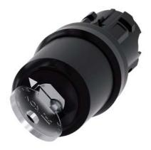
Key-operated switch IKON, 22 mm, round, plastic, lock number 360012K1, with 2 keys, 2 switch positions O-I, latching, actuating angle 90°, 10:30h/13:30h, key removal O, with laser labeling, upper case
