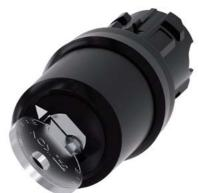
Key-operated switch IKON, 22 mm, round, plastic, lock number 360012K1, with 2 keys, 2 switch positions O-I, latching, actuating angle 90°, 10:30h/13:30h, key removal O, with laser labeling, upper case and lower case, always upper case at beginning of line
