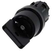
Key-operated switch O.M.R, 22 mm, round, plastic, lock number 73034, black, with 2 keys, 2 switch positions O-I, latching, actuating angle 90°, 10:30h/13:30h, Key removal O+I Z=50-unit packaging
