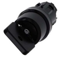
Key-operated switch O.M.R, 22 mm, round, plastic, lock number 73034, black, with 2 keys, 2 switch positions O-I, latching, actuating angle 90°, 10:30h/13:30h, key removal O, with laser labeling, inscription or symbol Customer-specific selection with SIRIUS ACT configurator (CIN)
