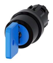
Key-operated switch O.M.R, 22 mm, round, plastic, lock number 73038, blue, with 2 keys, 3 switch positions I-O-II, latching, actuating angle  $2x45^{\circ}$ , 10:30h/12h/13:30h, key removal O, with laser labeling, lower case
