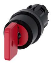
Key-operated switch O.M.R, 22 mm, round, plastic, lock number 73037, red, with 2 keys, 3 switch positions I-O-II, latching, actuating angle  $2x45^{\circ}$ , 10:30h/12h/13:30h, key removal O+I, with laser labeling, upper case and lower case, always upper case at beginning of line
