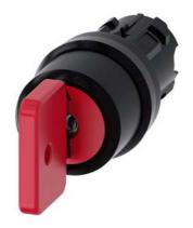
Key-operated switch O.M.R, 22 mm, round, plastic, lock number 73037, red, with 2 keys, 3 switch positions I-O-II, latching, actuating angle 2x45°, 10:30h/12h/13:30h, key removal O, with laser labeling, inscription or symbol Customer-specific selection with SIRIUS ACT configurator (CIN)
