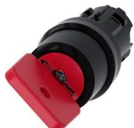
Key-operated switch O.M.R, 22 mm, round, plastic, lock number 73037, red, with 2 keys, 2 switch positions O-I, latching, actuating angle 90°, 10:30h/13:30h, key removal O, with laser labeling, upper case and lower case, always upper case at beginning of line
