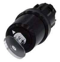
Key-operated switch BKS, 22 mm, round, plastic, Lock number E1 (VW), without key, 2 switch positions O-l, latching, actuating angle  $90^\circ$ , 10:30h/13:30h, key removal O, with laser labeling, upper case
