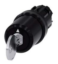
Key-operated switch BKS, 22 mm, round, plastic, lock number S1, with 2 keys, 3 switch positions I-O<II, left latching, right momentary contact type, actuating angle  $2x45^{\circ}$ , 10:30h/12h/13:30h, key removal I, with laser labeling, upper case and lower case, always upper case at beginning of line
