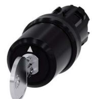
Key-operated switch BKS, 22 mm, round, plastic, lock number S1, with 2 keys, 3 switch positions I-O<II, left latching, right momentary contact type, actuating angle 2x45°, 10:30h/12h/13:30h, Key removal I Z=50-unit packaging
