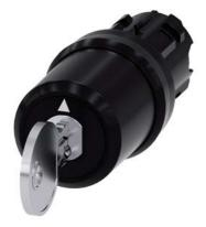
Key-operated switch BKS, 22 mm, round, plastic, lock number S1, with 2 keys, 3 switch positions I-O-II, latching, actuating angle 2x45°, 10:30h/12h/13:30h, key removal I, with laser labeling, inscription or symbol Customer-specific selection with SIRIUS ACT configurator (CIN)
