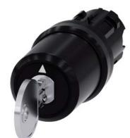
Key-operated switch BKS, 22 mm, round, plastic, lock number S1, with 2 keys, 3 switch positions I-O-II, latching, actuating angle  $2x45^{\circ}$ , 10:30h/12h/13:30h, key removal I, with laser labeling, lower case
