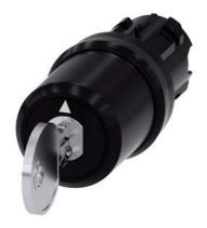
Key-operated switch BKS, 22 mm, round, plastic, lock number S1, with 2 keys, 3 switch positions I-O-II, latching, actuating angle 2x45°, 10:30h/12h/13:30h, Key removal I+O+II, with laser labeling, upper case and lower case, always upper case at beginning of line
