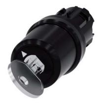
key-operated switch Siemens, 22 mm, round, plastic, lock no. LSG1, with 2 keys, 2 switch positions O-I, latching, actuating angle  $90^\circ$ , 10:30h/13:30h, key removal O+I, with laser labeling, upper case and lower case, always upper case at beginning of line
