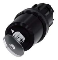
key-operated switch Siemens, 22 mm, round, plastic, lock no. LSG1, with 2 keys, 2 switch positions O<I, momentary contact type, actuating angle 45°, 10:30h/12h, key removal O, with laser labeling, upper case and lower case, always upper case at the beginning of the word
