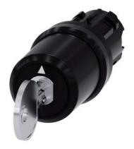
key-operated switch Siemens, 22 mm, round, plastic, lock number SSG10, with 2 keys, 3 switch positions I>O<II, momentary contact on the left, latching on the right, actuating angle 2x45°, 10:30h/12h/13:30h, key removal O+II, with laser labeling, inscription or symbol customer-specific selection with SIRIUS ACT configurator (CIN)
